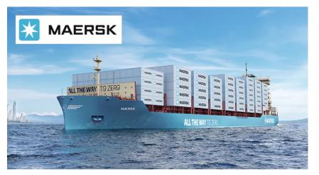
The use of heavy oil as a marine fuel is a key problem for shipping companies. Maersk is leading the way towards a solution and will soon operate the world's first container ship powered by green methanol.
